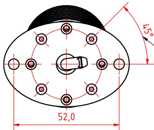
The 10° wedge can be reoriented in relationship to the base plate in 45° Intervals
