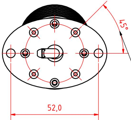
The 10° wedge can be reoriented in relationship to the base plate in 45° Intervals
