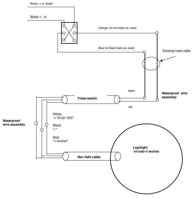
The standard non-waterproof switch can be replaced with any three-position, double throw-switch
