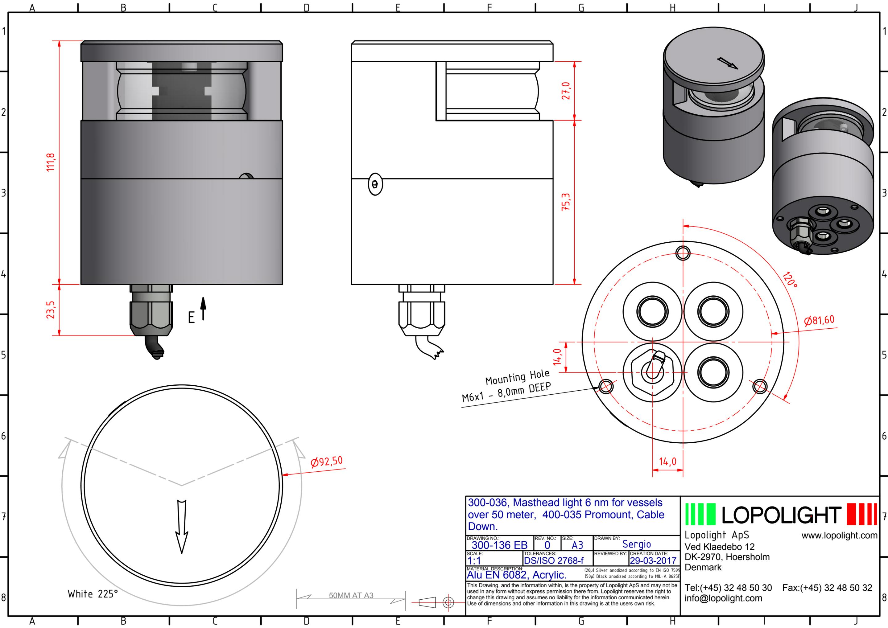
**300-036, Masthead light 6 nm for vessels over 50 meter, 400-035 Promount, Cable Down.**
