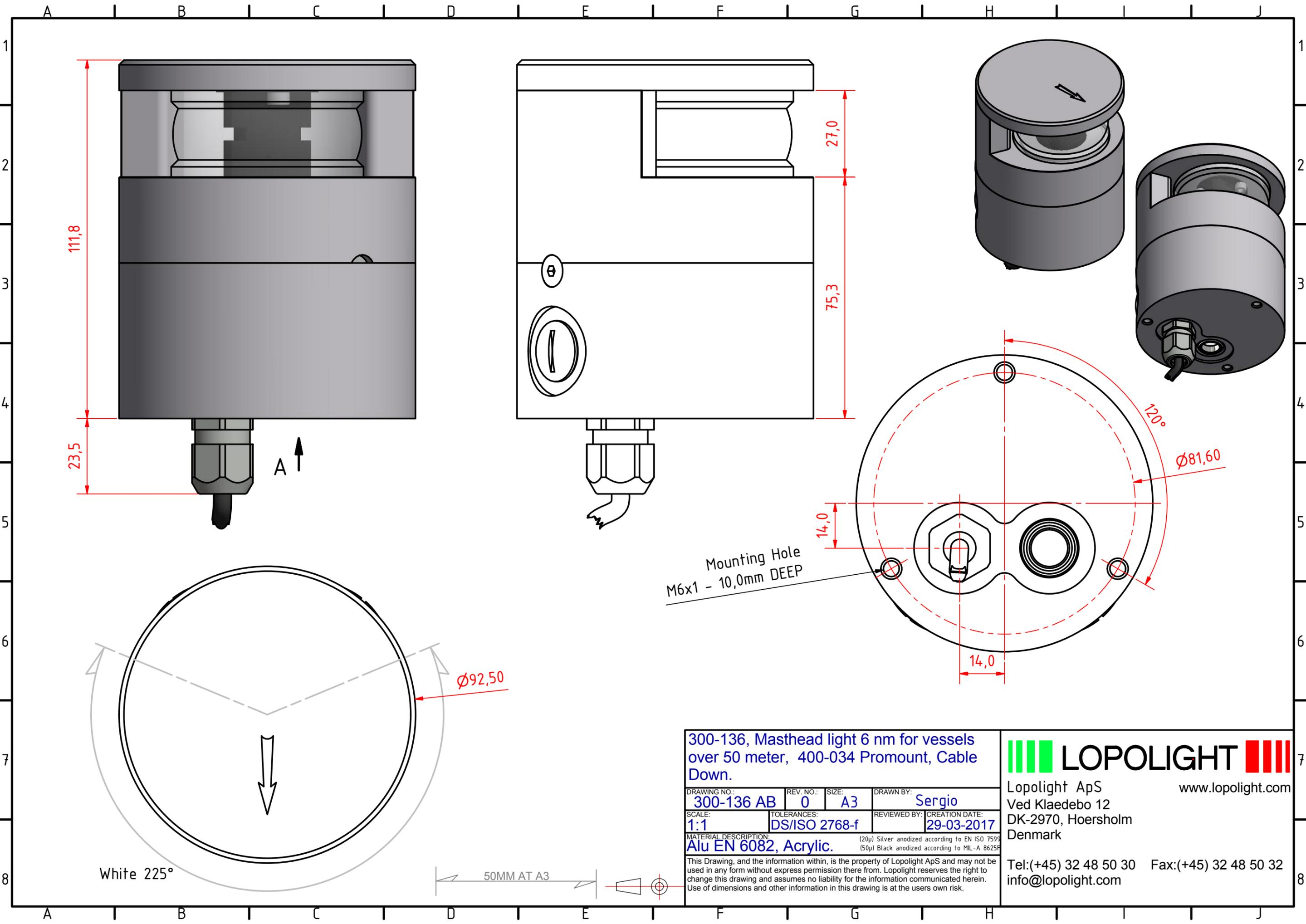
**300-136, Masthead light 6 nm for vessels over 50 meter, 400-034 Promount, Cable Down.**
