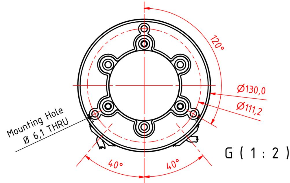
**300-136, Masthead light 6 nm for vessels over 50 meter, PRO-Series Promount, PE Base Plate, 2 Cable Side.**
