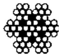
7 X 7 CONSTRUCTION 7 strands of 7 wires
