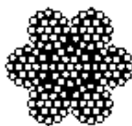
7 X 19 CONSTRUCTION 7 strands of 19 wires
