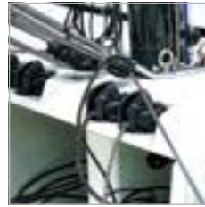
Carbon fibre cam C-Cleat™
