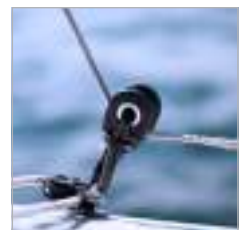
Cheek plates twist to open block
