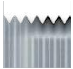
Rolled threads for maximum strength
