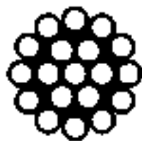
1 X 19 CONSTRUCTION 19 single strands
